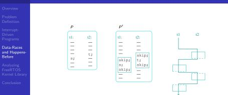
Figure: Illustrating the definition of a data-race on statements s and t. A program P, its transformation P', and an execution of P' in which the blocks overlap.
